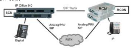
The SIP interoperability support between IP Office and BCM50/450 allows customers to migrate a network of BCM step by step to an IP Office SCN or Server Edition network.
