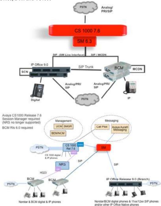
This configuration allows migrating a network of BCM and CS1000 to the IP Office step by step by adding IP Office systems to it.
