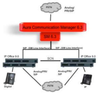
The SIP protocol is used for trunks between the IP Office nodes and the SM. The IP Offices are a network of SCNs and can use advanced SCN feature set between each other.
