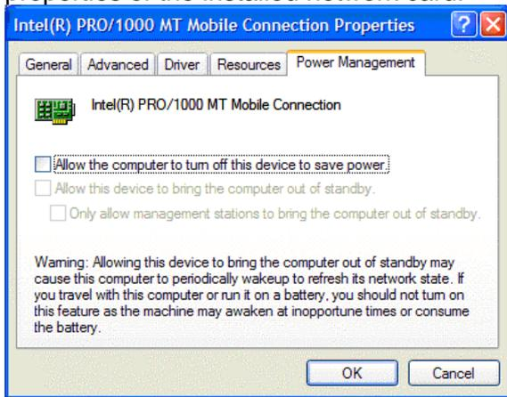
12. If the server PC is directly connected to the IP Office control unit, adjust the NIC port settings to match the IP Office as follows. If connected via a LAN switch, check the LAN switch manufacturers documentation for details of the optimum port settings.
