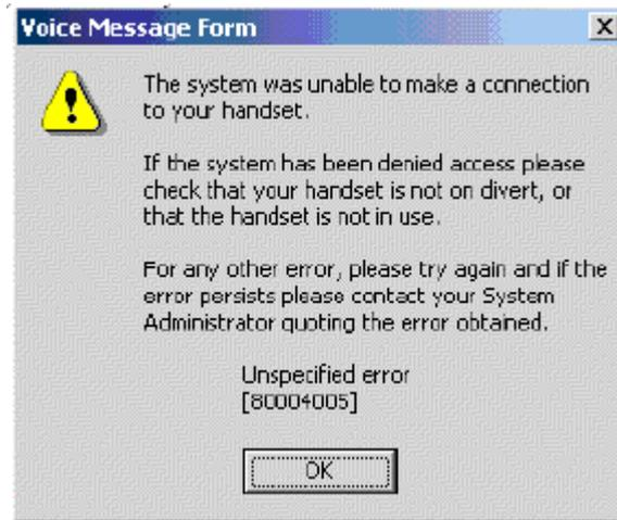
This error is typically only seen when selecting the handset as the Output device. If the message is embedded or attached a user can play the message using desktop speakers.
